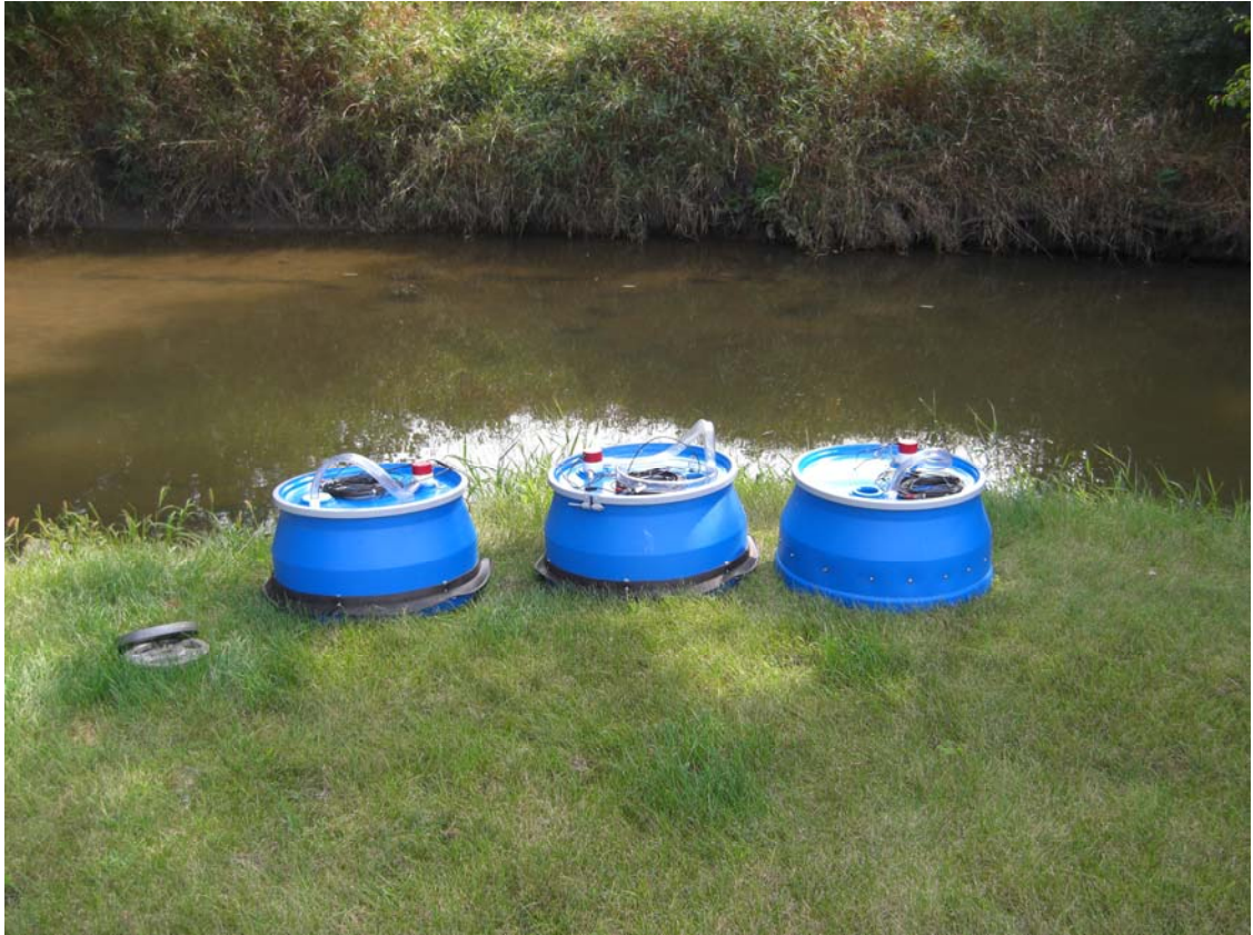
Figure 2-3 CDM Constructed SOD Chambers
